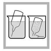
8. Prepare the sample: Collect at least 40 mL of sample in a 50-mL beaker. Fill a DPD Free Chlorine Reagent AccuVac Ampul or a DPD Total Chlorine Reagent AccuVac Ampul with sample. Keep the tip immersed while the AccuVac Ampul fills completely.
