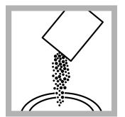
**9.** Add one 10-mL DPD Free Chlorine Reagent Powder Pillow or one 10-mL DPD Total Chlorine Reagent Powder Pillow to the second sample cell.
