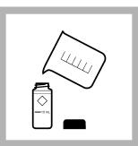
**2. Prepare the blank:** Fill a sample cell to the 10-mL mark with sample. Close the sample cell.
