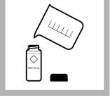
**8. Prepare the sample:** Fill a second sample cell to the 10-mL mark with sample.
