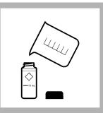
**2. Prepare the blank:** Fill a sample cell to the 10-mL mark with sample. Close the sample cell.
