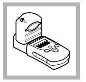
**5.** Install the instrument cap over the cell holder.
