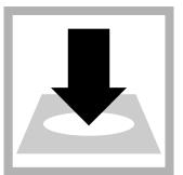
**14. Total chlorine measurement:** After 3 minutes and within 6 minutes of the reagent addition, insert the prepared sample into the cell holder. Point the diamond mark on the sample cell toward the keypad.
