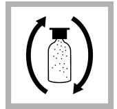
**9.** Quickly invert the AccuVac Ampul several times to mix.
